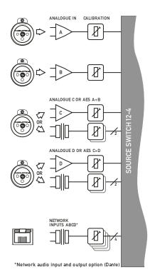
Your amplifier can source audio from analogue, AES digital, or network locations (if a network card is fitted).
