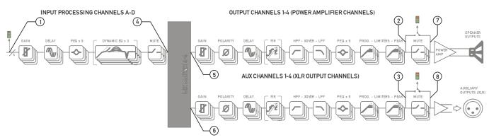
If your amplifier has a network audio card fitted (Dante) then, as well as being able to route four channels of audio from the network, it is possible to route four channels of audio back onto the network. The possible sources for the network outputs are always selected as a group of four, and there are eight points within your amplifier's DSP than can be chosen.
