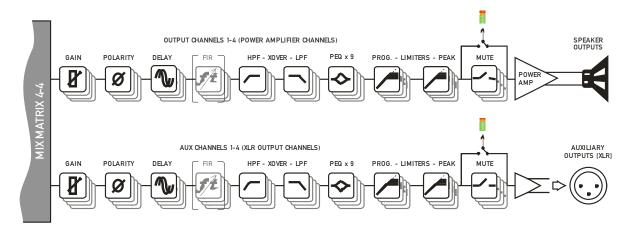
There are eight identical channels of output processing in your amplifier: four dedicated to the power amplifier channels, and a further four that are connected to the auxiliary XLR outputs on the amplifier, providing analogue feeds to other equipment.
