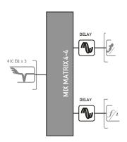
The mix matrix allows four independent mixes to be set up for the power amplifier channels and the auxiliary output channels.
