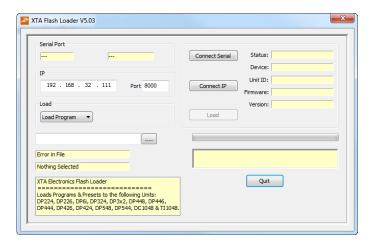
Press the "Connect Serial" button if using USB or RS485, or "Connect IP" if using an Ethernet connection. We recommend you choose either a USB or wired Ethernet connection.
