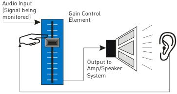
Feedback Path from Monitor Engineer's Ears to Hand forming Sidechain Control Signal
