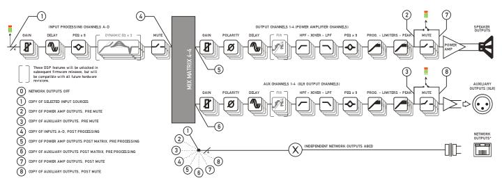
If your amplifier has a network audio card fitted (Dante) then, as well as being able to route four channels of audio from the network, it is possible to route four channels of audio back onto the network.
