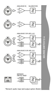
Your amplifier can source audio from analogue, AES digital, or network locations (if a network card is fitted).
