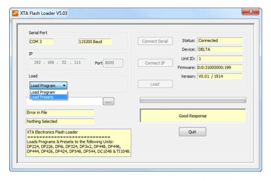
The file type will have been filtered for you – LTAM\*.bin for firmware (program) files or LTAR\*.bin for preset files.
