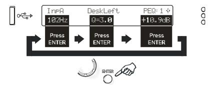
Finally, use the rotary encoder to adjust the value of the parameter.
