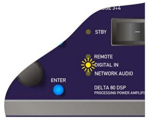
Note that the AES LED being illuminated does NOT mean that an AES source is being used or routed anywhere within the amplifier. It is an indication that valid AES is connected. If the AES input(s) have valid stable signals and there are no other issues, the LED will not be flashing.
