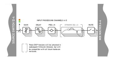
Your amplifier has four input channels of processing that can be fed from a variety of sources.
