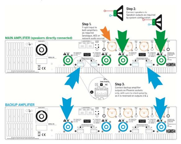
Step 1: Connect both amplifiers inputs to the required sources and make sure both amplifiers are configured the same for routing, and source (analogue/AES/network).
