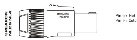
Additionally, Channel 1 Speakon connector carries Channel B2output on Pins +2 & -2 to allow easy bi-amping or bridged operation using a single NL4 connector. Similarly, Channel 3's Speakon connector also carries Channel 4 output.
