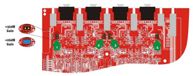
Remember, setting higher gain does not change the maximum available power but changes the level of signal input to achieve maximum power. In any case, provided that the input signal is less than 20dBu/7.7V, the built in limiter circuit will prevent distortion within the amplifier.
