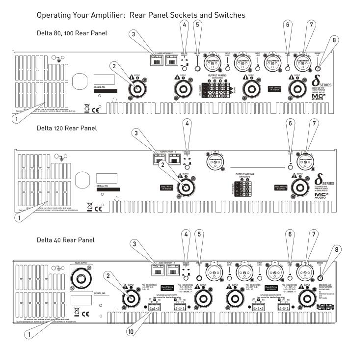
1: Fan outlet: The variable speed fans suck air in through the front vents and out through the back of the amplifier. Please see maintenance on page 19 for recommendations on how to clean this and the front foam sections.
