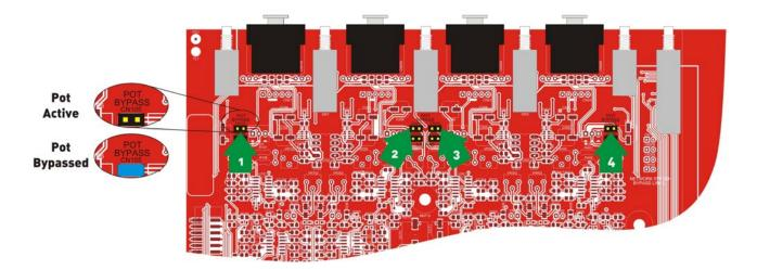
Adding a link to CN105 disables the pot for channel A, CN205 disables the pot for channel B, and so on.
