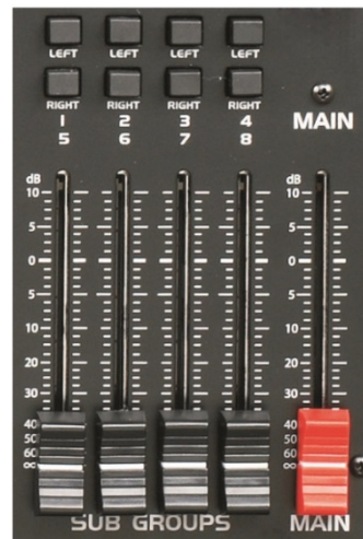
Fig. 4.18 Subgroups and main mix fader
