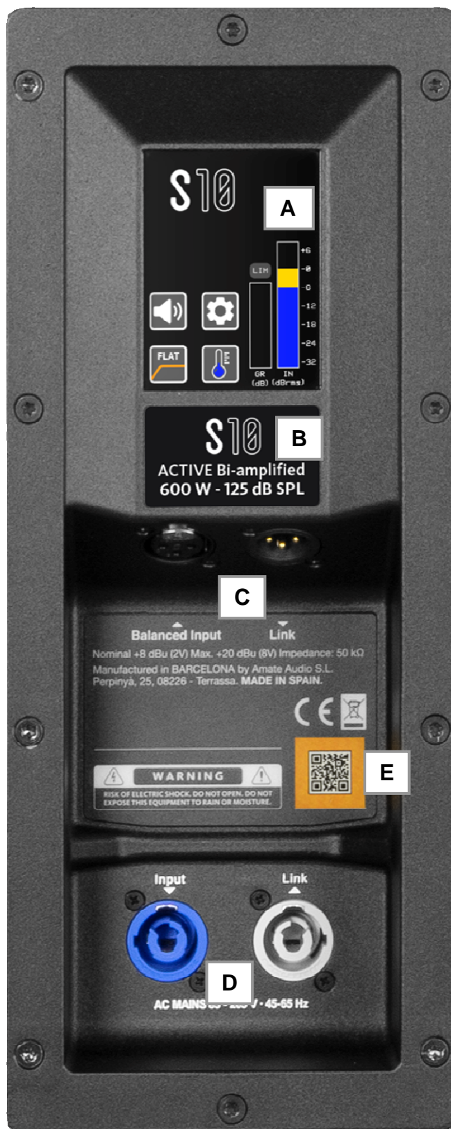
Fig. 2. S10 control and connection panel
